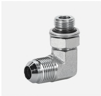
P/N:1JH9-OG 90°elbow JIC male 74°cone /metric adjustable stud end I-series
